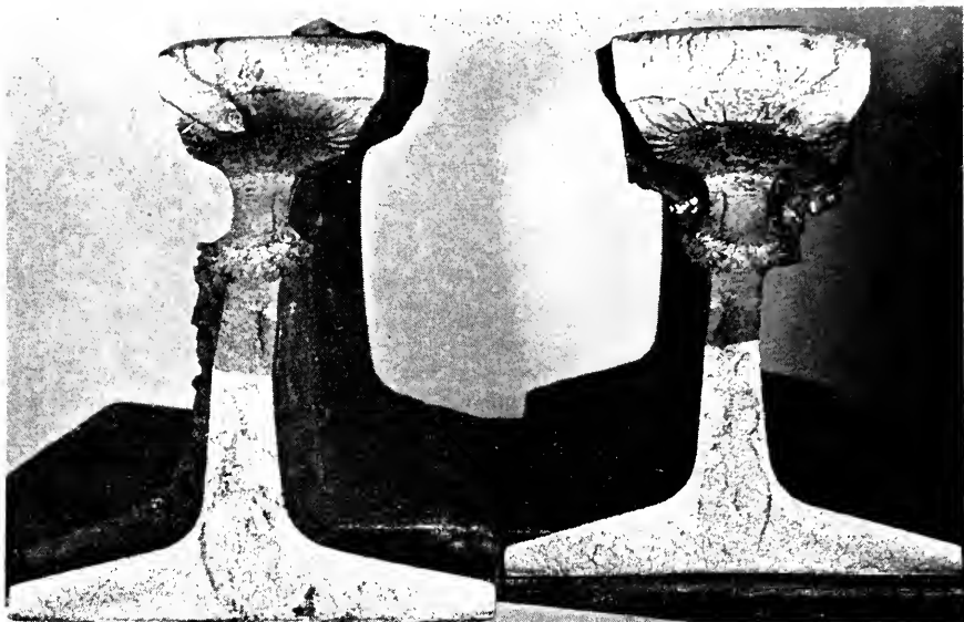
Fig. 9—Fractured faces of an electric flash butt welded rail joint, specimen 226A, that failed after being subjected to 1,682,100 cycles of repeated loading in the 12-in-stroke rolling-load machine under a 57,500-lb wheel load. It can be noted that a pipe is present in the web of these rails, but an analysis of the fracture mechanics indicates that this failure originated in the fillets between the web and upset metal.
